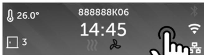
To access to the different panels, touch the related icon. Each panel can control a specific parameter of the air curtain.
