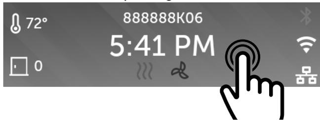
To access to the different panels, touch the related icon. Each panel can control a specific parameter of the air curtain.
